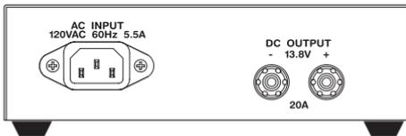
4. Insert the device's positive wire (usually red) into the red binding post's wire hole, then tighten the binding post's sleeve to secure the wire in place.
