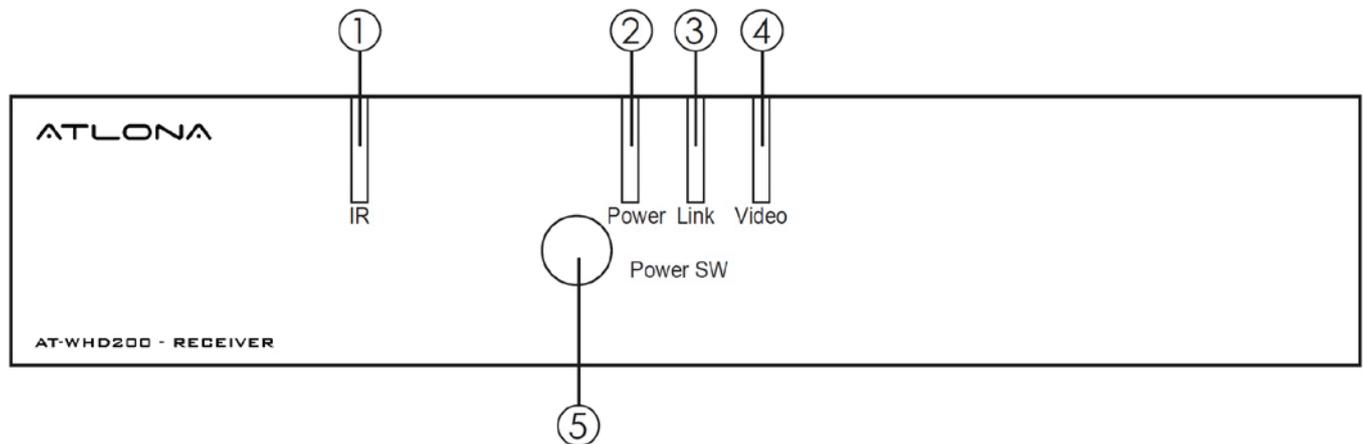
1. IR – IR receiver for remote signal to control the input source equipment.
