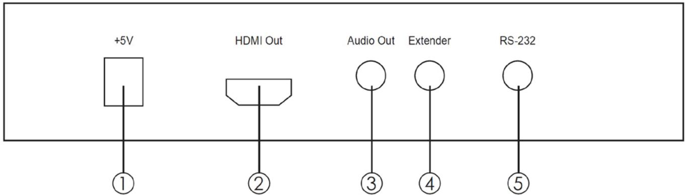
1. +5V – Power jack for plugging the adaptor from the power source.
