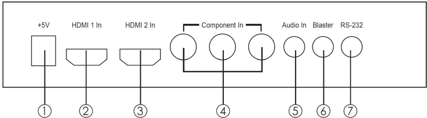
1. +5V – Power jack for plugging the adaptor from the power source.
