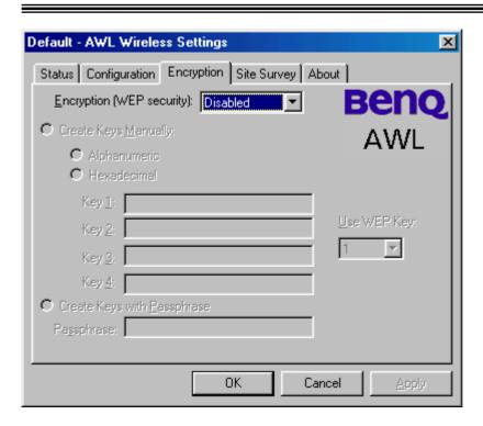
According to WEP function select, this page allows the entry of four keys for 64-bit and 128-bit encryption. Each key must consist of hex digits to be written to the driver and registry. This means that only digit number 0-9 and letters A-F are valid entries. Therefore, if entered incorrectly, the program will not write keys to a driver. You can also use Alphanumeric or Passphrase to create keys.
