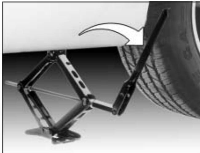
4. Raise the vehicle by turning the jack handle clockwise. Raise the vehicle far enough off the ground for the compact spare tire to fit underneath the wheel well of the vehicle.
