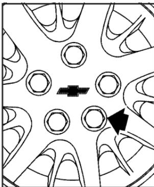
To remove the steel wheel covers and wheel nut caps, loosen the plastic nut caps with the wheel wrench in a counterclockwise direction. If needed, you can finish loosening them with your fingers. The plastic nut caps will not come off.
