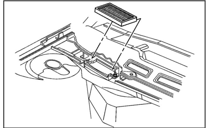
5. Remove the air inlet grille retainers.
