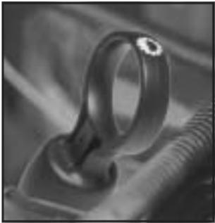
The transaxle fluid dipstick handle is the black loop near the rear of the engine compartment, toward the center. See *Engine Compartment Overview* on page 5-12 for more information on location.
