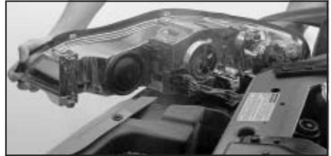
4. Pull the headlamp assembly away from the vehicle and remove the electrical connector.
