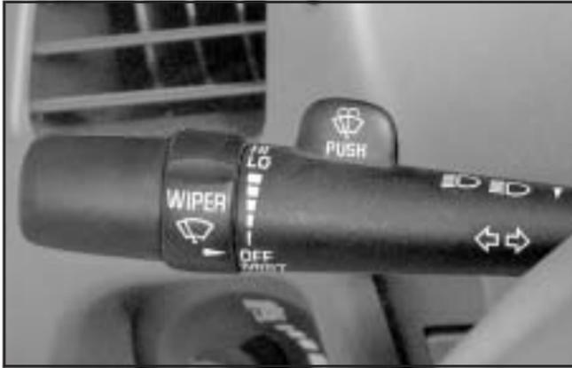
The windshield wipers will operate when the ignition is in ACC or ON.
