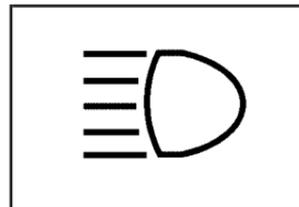
This light will illuminate when the headlamp high beams are in use.
