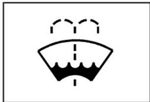
Open the cap with the washer symbol on it. Add washer fluid until the tank is full. See *Engine Compartment Overview* on page 5-12 for more information on location.
