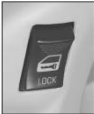
A power door lock switch is located on each front door above the armrest.
