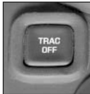
To turn the system on or off, press the TRAC OFF button on the console.
