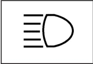
While the high beams are on, this light will appear on the instrument panel cluster.
