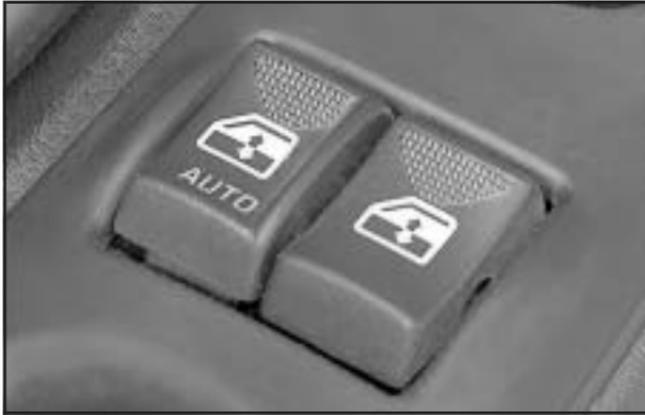
Both doors have power window switches located on the armrest. Press the front of the switch to raise the window. Press the back of the switch to lower it. The switches on the driver's door armrest control each of the windows when the ignition is in ON, ACC, or when Retained Accessory Power (RAP) is active. See *Retained Accessory Power (RAP)* on page 2-17.
