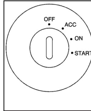
The ignition switch is located on the instrument panel, to the right of the steering column.
