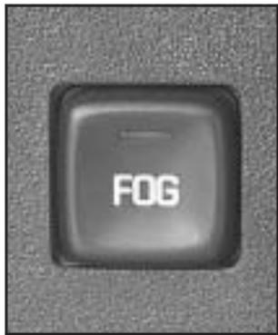
If your vehicle has this feature, the fog lamp button is located on the instrument panel, next to the exterior lamp control wheel, to the left of the steering column.
