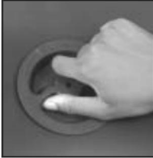
1. Turn the center nut on the compact spare tire cover counterclockwise to remove it. Then remove the cover.
