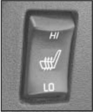
If your vehicle has this option, the switches that control seat temperature are located on the center console.
