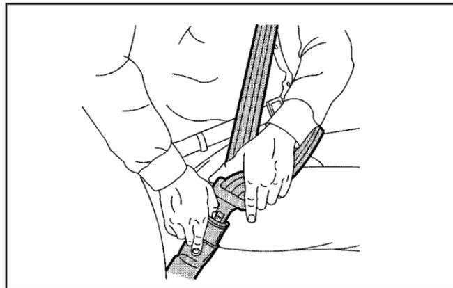
To unclatch the belt, just push the button on the buckle.
