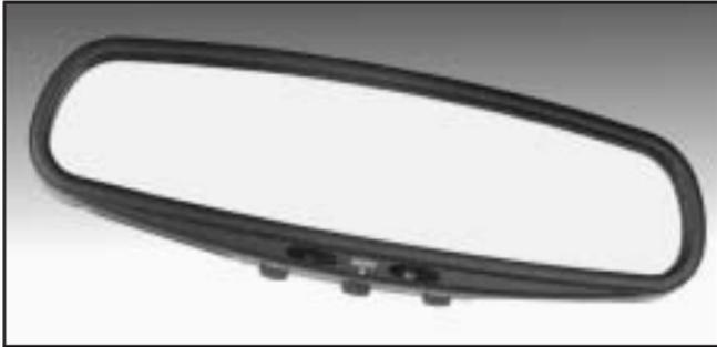
The vehicle may be equipped with an automatic dimming rearview mirror. Push the center button on the bottom of the mirror to turn this feature on. The mirror will darken gradually to reduce glare from headlamps behind you. This may take a few moments. The mirror will lighten whenever you shift to REVERSE (R).
