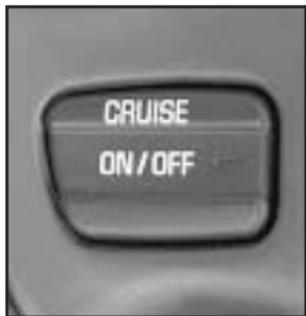
1. Push the CRUISE ON/OFF button located on the steering wheel to turn the cruise control on.
