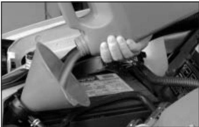
5. Fill the radiator with the proper DEX-COOL<sup>®</sup> coolant mixture, up to the base of the filler neck. See *Engine Coolant on page 5-29* for more information about the proper coolant mixture.
