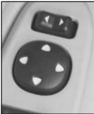
The outside power mirror controls are located near the driver's side window, on the armrest.
