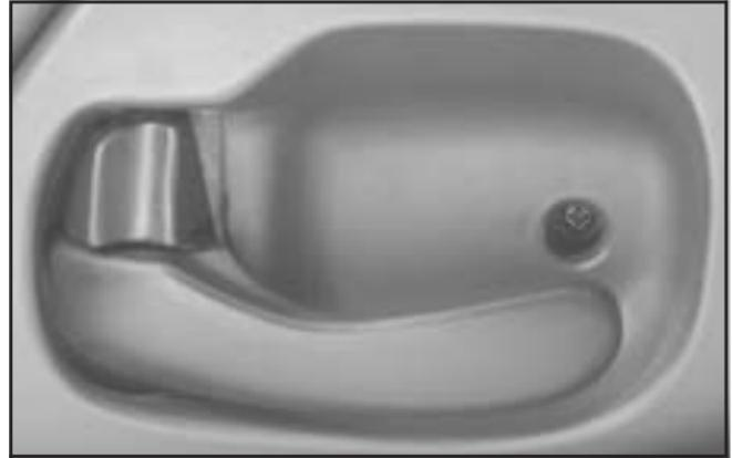
To lock a door from the inside, push the manual lock lever forward. To unlock a door, push the lever rearward.
