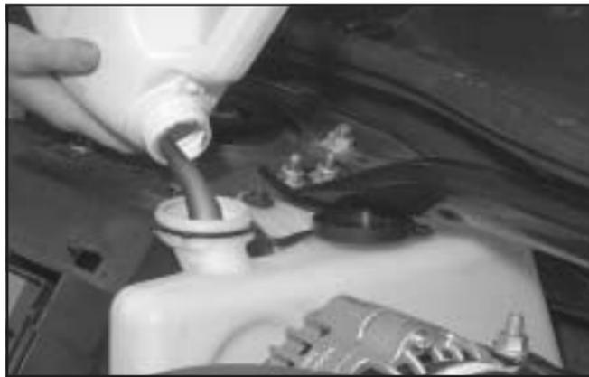
8. Then fill the coolant recovery tank to the COLD mark.
