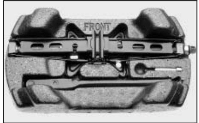
3. Turn the nut holding the jack counterclockwise and remove it. Then remove the jack and wrench.
