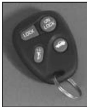
Using the remote keyless entry transmitter, you can lock and unlock your trunk doors or release your trunk from about 3 feet (1 m) up to 30 feet (9 m) away.
