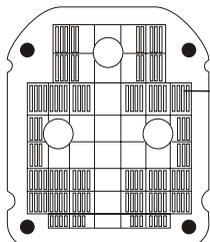
Ventilation hole at the bottom of the spin dryer
