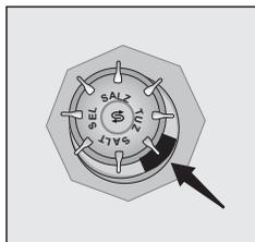
When this indicator light comes on, you must refill special salt. Only use special dishwasher salt in your machine to soften the water.
