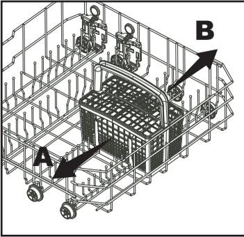
dishes according to their size, the Sliding Cutlery Basket can slide over the tines to the left **A** and right **B** side.
