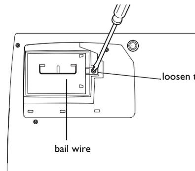
loosen the screw on lamp module
