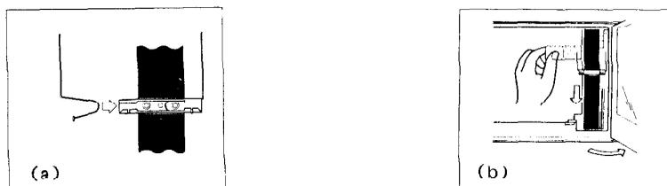
Fig.26 (a) Mounting the Stylus onto the Holder (b) and Rounding the Nib of the Stylus
