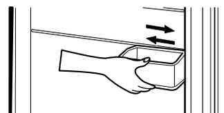
2. To remove the Design-A-Door bin, lift up from the bottom of the bin unclicks and pull straight out.
