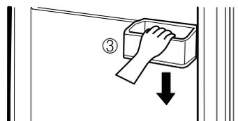
4. Make sure that if all bins are correctly assembled so that they don't fall out of door.
