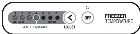
**NOTE:** Pressing OFF control key, we setting the refrigerator for exhibition mode. Only the refrigerator lights will work, not the refrigerator
