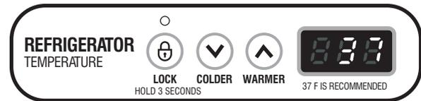
**NOTE:** You can lock the controls so the settings cannot be changed.
