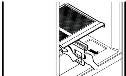
**WARNING:** Be careful when handling glass cover since glass is not attached to cover
