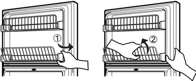
2. To replace the Freezer Door Bin, hook the end of the Door Bin in the bracket (1), then push down until the Door Bin locks into place (2).
