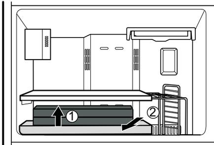
1. To remove the Flexi-Floor tray, lift slightly (1) and pull out towards you (2).
