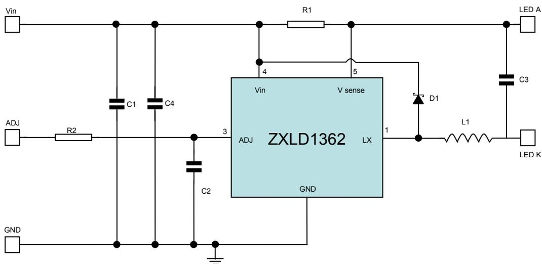
Figure 2: Schematic for the evaluation board ZXLD1362EV3
