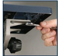
2. Secure the work table to the table trunnion using the four hex bolts and star washers (i).
