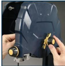
11. If required, adjust the saw blade tracking.
