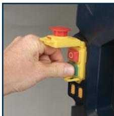
2. To switch off, simply push on the red cover (1) to snap it shut. This pushes the OFF button underneath the cover and cuts off the power. To switch on again it is necessary to unclip the cover and raise it.
