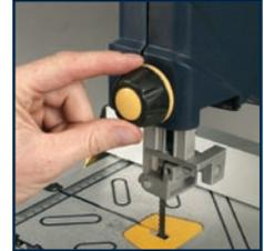
4. The upper blade guide consists of a thrust bearing that supports the band saw blade from the rear and two guide pins that provide lateral support, these need to be readjusted after every band saw blade change or tracking adjustment.
