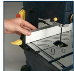
4. Attach the rip fence to the table and secure it by pushing down the rip fence locking handle (29).
