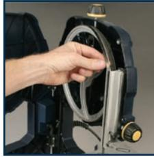
6. Remove the blade by guiding it through the slot in the work table and the upper and lower blade guides.
