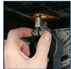
2. Press the guide pins together against the band saw blade.
