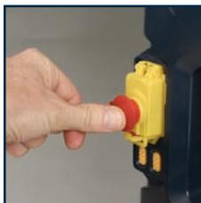
**Note.** The saw is automatically turned off in the event of a power failure. You will need to press the ON button again to restart the saw.
