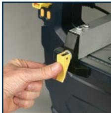
3. Ensure that the fence rests against the wood along its entire length to give a consistent parallel cut.
