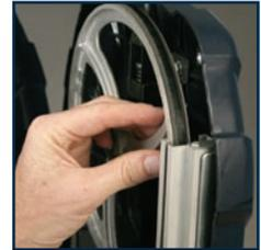
2. Adjust the thrust bearing position until it is 0.5mm away from the band saw blade. When the band saw blade is turned by hand it should not make contact with the thrust bearing.
