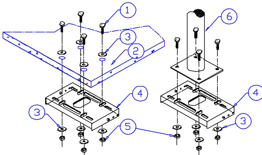
**NOTE:** If ASA-2446 adjustable height suspension adapter is a part of the installation, securely install the adapter to the ceiling at this time (see detail above)
