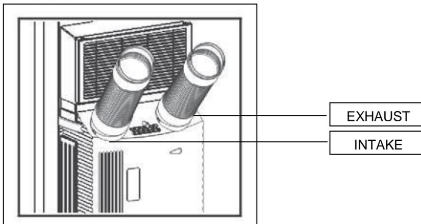
4. Only extend the exhaust hoses to the necessary length. We do not recommend extending the exhaust hose more than 9' long. Additional 4' exhaust hose sold separately.
