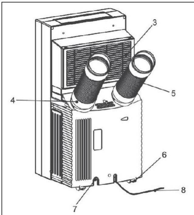
3. Evaporator air intake / air filter
