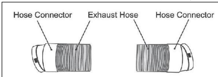
3. Align the slots on the hose connector to the tabs on the air intake / outlet and snap the hose to the unit.
