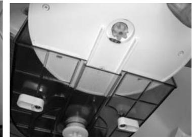
Aluminum/auger mixing mechanism in mixing chamber, and being lifted out
