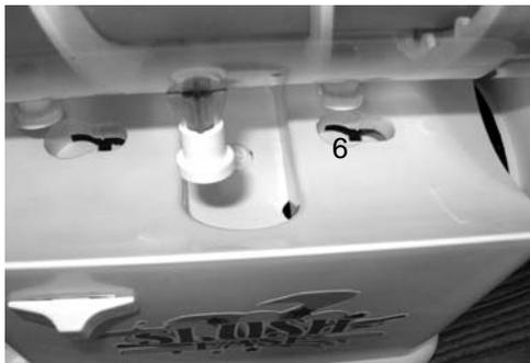
4. Pull the 2 white end plugs (front and back) out to release the aluminum/auger mixing mechanism from mixing chamber. (See Illustration)
