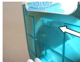
14. Pour beverage into unit. DO NOT fill Past fill line. NOTE: Be sure to use sugar based beverages. (Sugar substitute drinks do not freeze well – such as diet drinks.)
