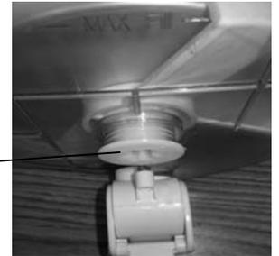
5. Lift out the aluminum/auger mixing mechanism from mixing chamber. (See Below)
