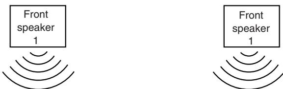
Use front speakers with 8 Ω – 16 Ω impedance.
