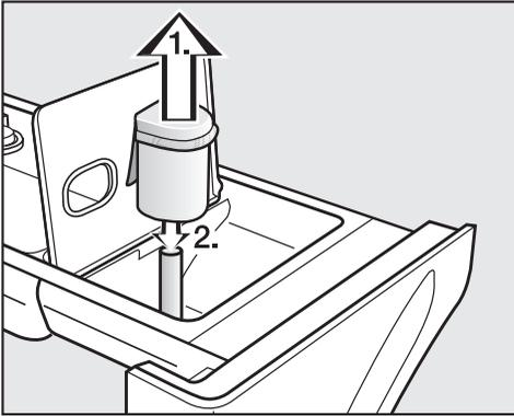
1. Remove the siphon from compartment
