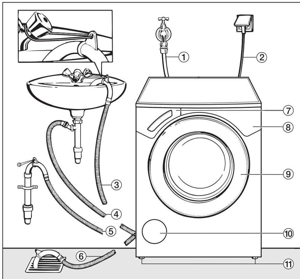
① Inlet hose (tested to withstand pressure of at least 7,000 kPa)
