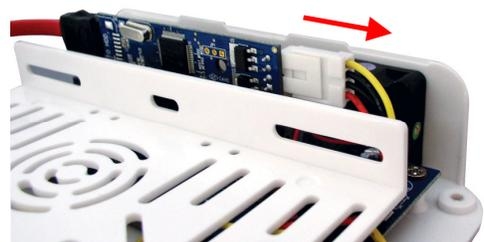
7. Disconnect the SATA Data cable from the bridgeboard. Hold the base of the drive enclosure and pull the bridgeboard up to disconnect it.
