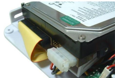
12. Use the supplied screws to secure both sides of the drive
