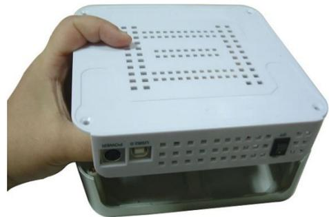
14. Replace the 4 case screws and affix the two foam feet as illustrated
