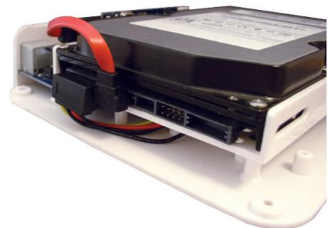
5. Before you can connect your IDE hard drive you must first remove the SATA Bridge Board and Molex to SATA power cable.
