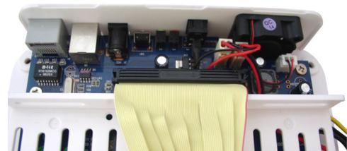
11. Place the hard drive into the drive tray and connect the Molex power and IDE data cables
