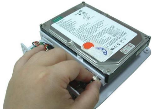
13. Carefully assemble the top and bottom of the case. If the upper case does not fit properly, adjust the hard disk position and try again
