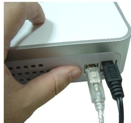
**Note:** If you are using the FireWire interface, you can plug the cable into either of the FireWire sockets. The second socket can be used for connecting another FireWire device in series.
