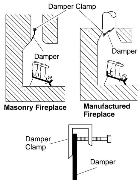
Figure 5 - Attaching Damper Clamp
