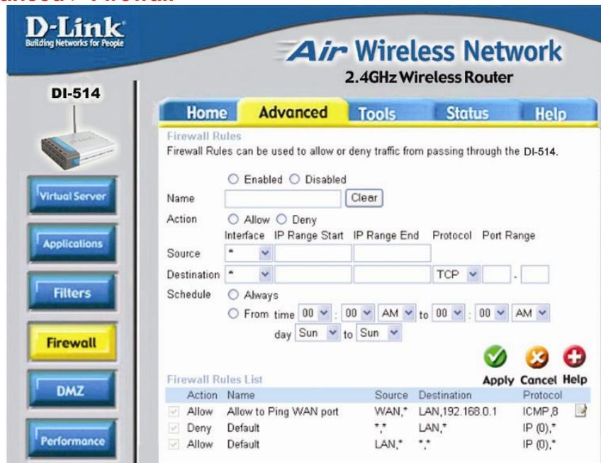
Firewall Rules is an advance feature used to deny or allow traffic from passing through the Broadband Router. It works in the same way as IP
