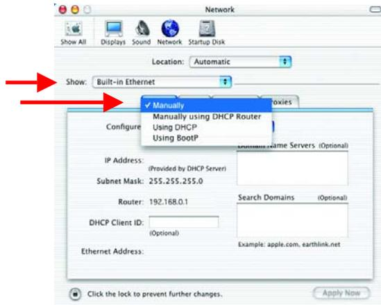
Input the **Static IP Address**, the **Subnet Mask** and the **Router IP Address** in the appropriate fields.
