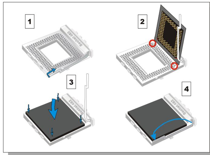
1. Lift the socket handle up to a vertical position.
