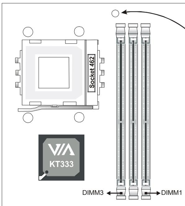
To avoid shorting the motherboard to the case, please use the provided spacer support on this screw hole...
