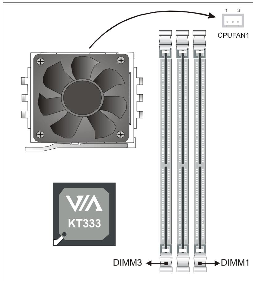
**Note:** If the fan is defective or power connector is not connected to CPUFAN1, the system will enable Fan Off Control function. See below for more information on FOC function.
