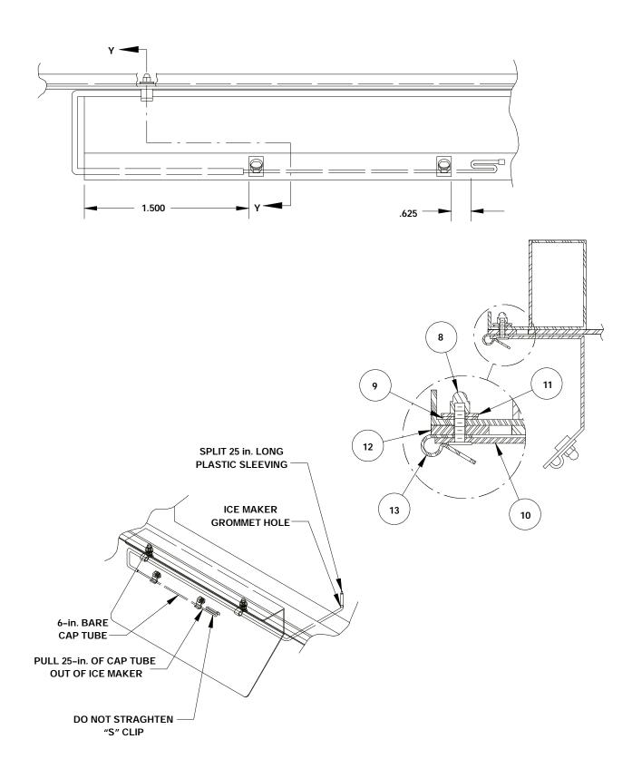
FIGURE 3. CAPILLARY TUBE LOCATION
