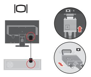
Connect the digital signal cable to the video port on the back of the computer.  $\mbox{\bf Note} :$  One end of the signal cable is already pre-attached to your monitor.
