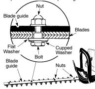
1. Using a wrench, loosen each nut on the top side of the blade guide.
