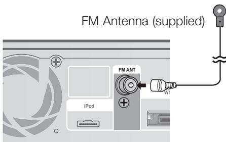
1. Connect the FM antenna supplied to the FM 75Ω COAXIAL jack.
