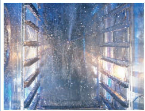
**air-o-clean:** Integrated automatic self-cleaning system. Hassle-free cleaning of air-o-speed™ after use.
