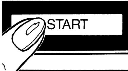
**Step 4:** Touch START. Inside light comes on and fan starts. Cooking time counting down shows on display.
