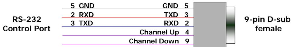
RS-232 wiring for control or programming should only use pins 2, 3, 5. Cables with all pins wired can lock out front-panel programming and data communication (Pins 4 and 9 are inputs).
