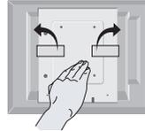
Do not remove the tape with the set up side down as the <Image 2>. The base part may spring up to injure your hand.
