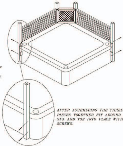
AFTER ASSEMBLING THE THREE PIECES TOGETHER FIT AROUND SPA AND TOE INTO PLACE WITH SCREWS.
