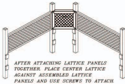
AFTER ATTACHING LATTICE PANELS TOGETHER. PLACE CENTER LATTICE AGAINST ASSEMBLED LATTICE PANELS AND USE SCREWS TO ATTACH.
