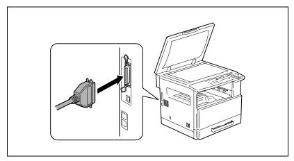
This completes connection of the machine to the computer.
