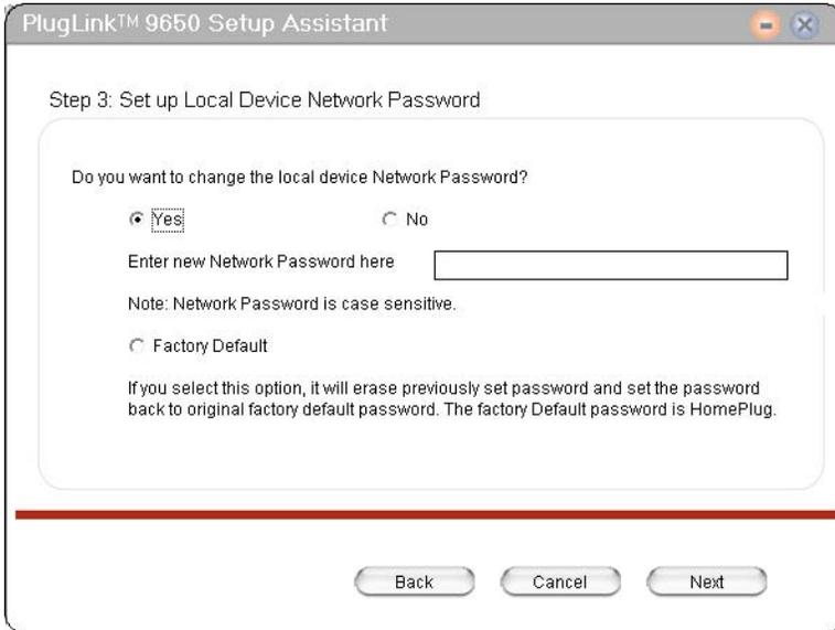
*Figure 6-5: Local Device Network Password Screen.*
