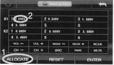
5.(1)press the button step by step on car steering wheel control and write it down,then click "allocate" button on our unit like as picture show
