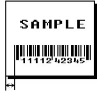
**NOTE:** Allow a minimum of **1/10** inch between the scan edge of bar code and label edges or other data.
