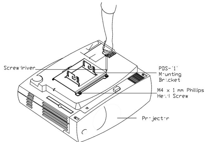
1. Invert the projector and place it on a soft and flat surface. Remove any foot levelers that might possibly prevent the correct installation of the bracket.
