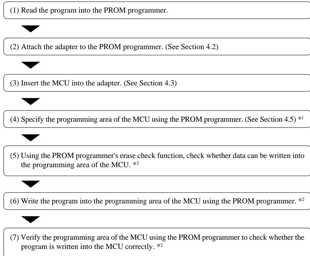
\*1 **Be sure to set the programming area. Otherwise the mode's shift to the programming mode may not be performed successfully. The erase check function etc. may not also be performed completely.**
