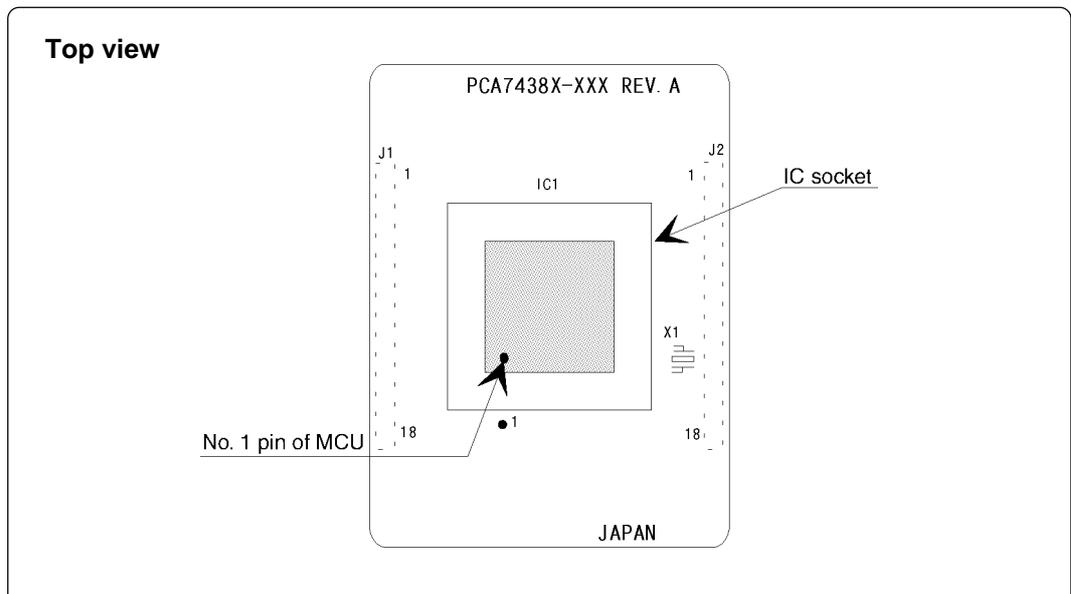
Figure 4.2 Inserting an MCU
