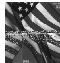
Comparison of DCDi deinterlaced (progressive scan) output (top) with conventional progressive scan processing (bottom). Proprietary Faroudja technology identifies moving images at all angles, and uses exclusive algorithms to process the moving edges, producing a smooth image that is far more film-like than is possible with conventional progressive scan processing. DCDi processing also eliminates coloration artifacts resulting from the deinter-lacing process.
