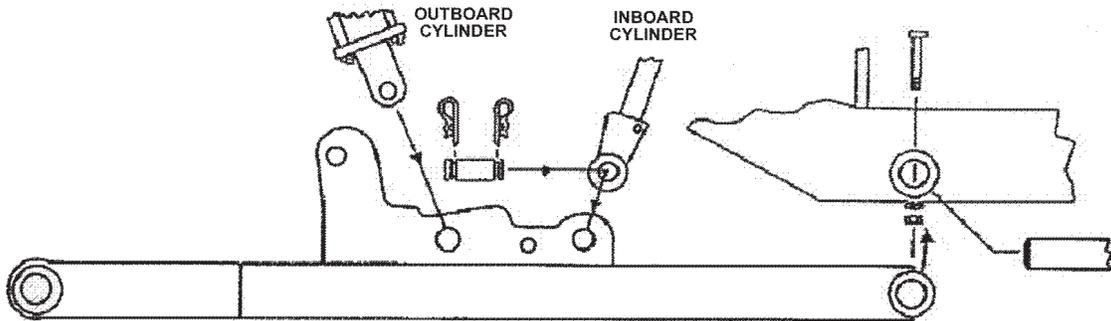
Install the fittings in the butt end of the outboard cylinder, as shown in the parts section. These should be positioned to face the rod end of the cylinder. Next, install the O-ring breather in the rod end of the cylinder.
