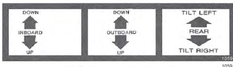
The rear mower height is controlled with the 3-point hitch control lever. Follow the instructions for this control in the tractor operators manual. The tilt of the rear mower is controlled with the third spool if the lift valve and is coordinated as shown above.
