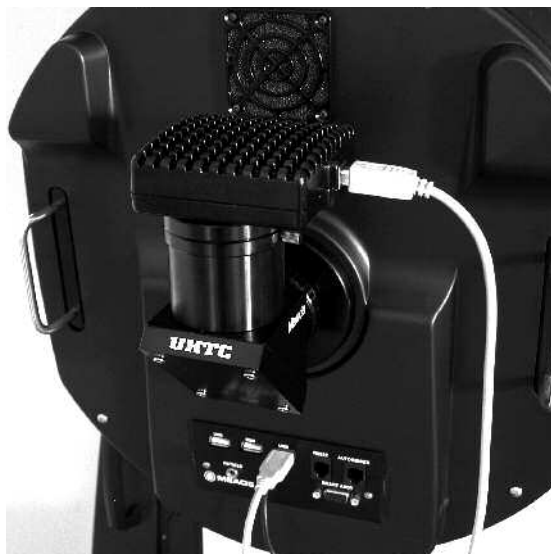
Fig. 38a: The Deep Sky Imager connected to the RCX400 diagonal mirror.
