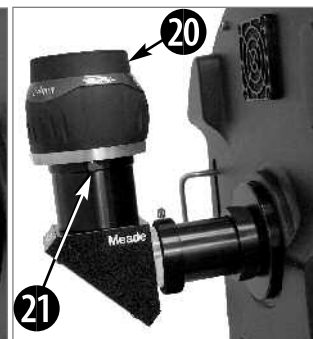
Fig. 20: Slide eyepiece (20) into the diagonal mirror and tighten thumbscrew (21).
