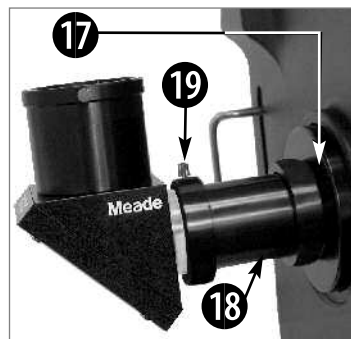
Fig. 19: Thread the ring of the visual back (18) onto the rear cell (17). Slide diagonal into the visual back and secure with thumbscrew (19).
