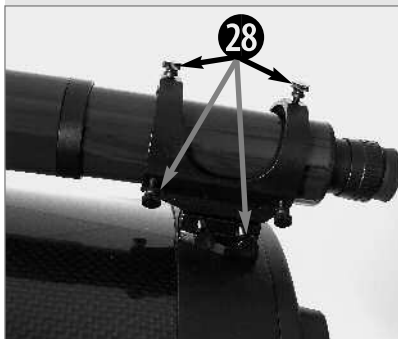
Fig. 23: Viewfinder adjustment screws (28).
