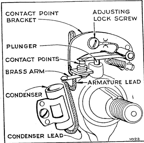
37. **TO REPLACE CONDENSER.** A leaky or weak condenser may cause the motor to start hard, to sputter or misfire under load. If motor misfires after checking gasoline line, carburetor, spark plug, cable and contact points, install a new condenser. Both the condenser lead and armature lead must be soldered to brass arm, see plate No. 10. Be sure to push condenser lead down between condenser and hub of magneto plate so it cannot rub against flywheel.
