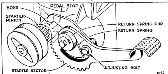
the bolt. Too much tension may cause spring to break. Be sure the spring is in the proper position with the long end below the pedal adjusting bolt and the hooked end in the slot of the cup.
