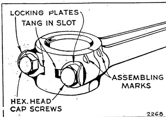
sembly marks on the lower bearing must be toward the magneto side. The assembly marks on cap and rod must be on the same side. On motors after serial No. 108719, place locking plate tang in slot and bend locking plates against hexagon head. See plate No. 13.
