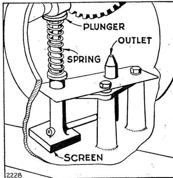
53. **OIL LEAKS.** If oil leaks from either end of crankshaft, remove base plate from motor. Oil return valves are screwed into crank case and magneto back plate at base of main bearings. Remove oil return valve and clean or flush with gasoline and blow out any dirt lodged under the small disc. See plate No. 9.
