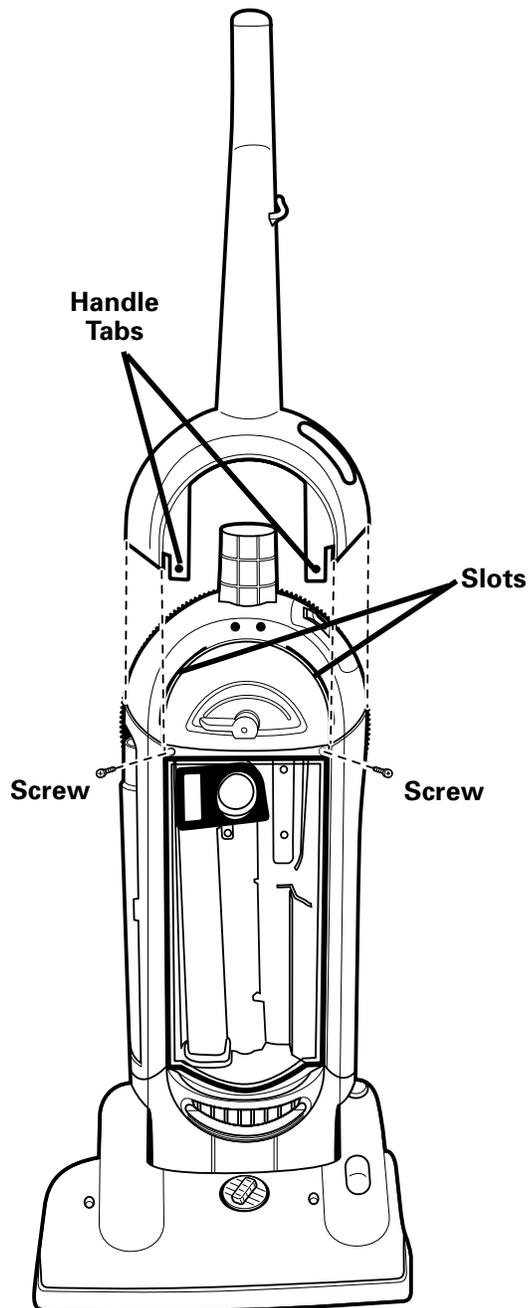
2. Position handle as above. Slide the handle down over the top of the unit, inserting handle tabs into slots on unit.
