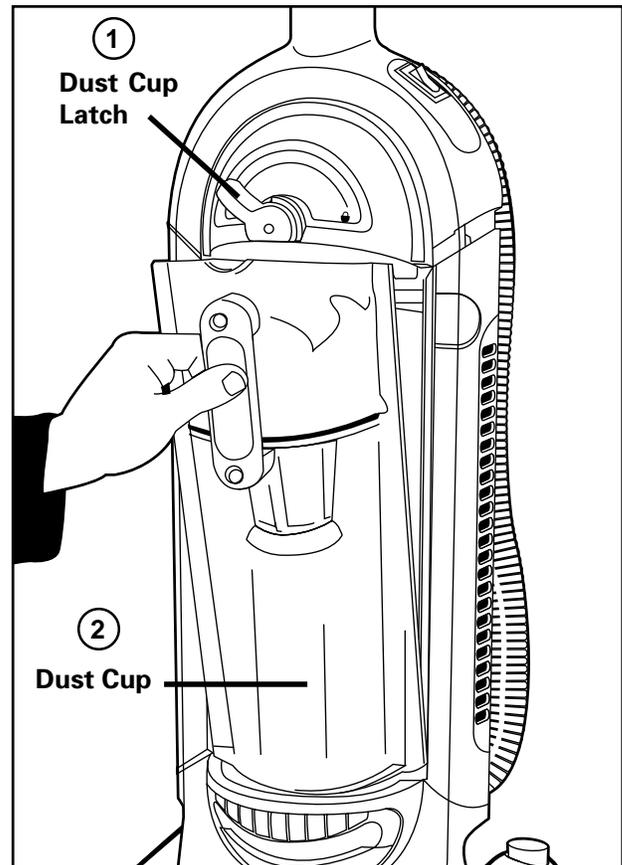
Release dust cup by rotating dust cup latch to the left pointing to the unlock symbol (⊕). Pivot dust cup out and away from cleaner and remove.
