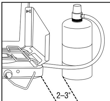
**NOTE:** Propane canister should be positioned a minimum of 2-3" from stove. Always use a canister with a flat bottom.
