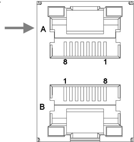
For a Gigabit Ethernet (10/100/1000) connection the network cable should be a CAT5 or above and include all four pairs.
