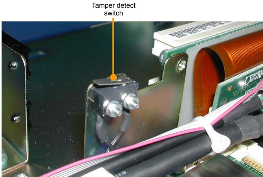
A tamper detection input is included within the real time clock circuitry of the APOLLO that operates in all power modes. The status of the tamper detection bit is battery backed in static RAM. Using a normally open switch, a tamper is detected when the switch contacts close.
