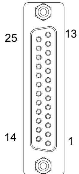
*J7B and J7C – COM1 and COM2 RS232 serial ports*
