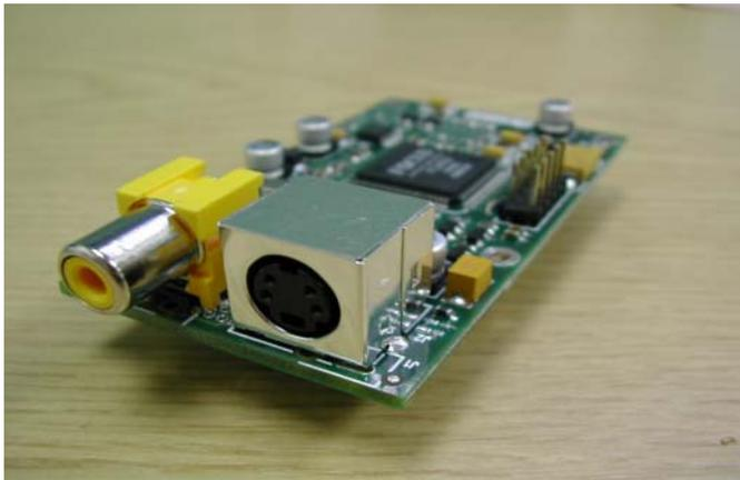
The TV Card converts APOLLO high-resolution DVO (Digital Video Output) from VGA to SXGA resolutions, and produces standard analog television (SDTV) output to S-Video and composite video connector outputs. The following image shows the TV card in position:
