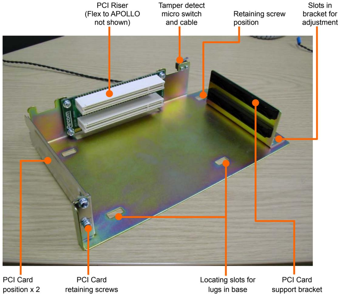
Remove any cables attached to installed PCI expansion cards before attempting removal of the PCI module.
