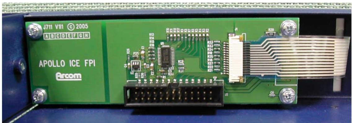
The Front Panel Interface is 'stacked' on the back of the LCD and has the tail from the front membrane plugged into a ZIF socket.
