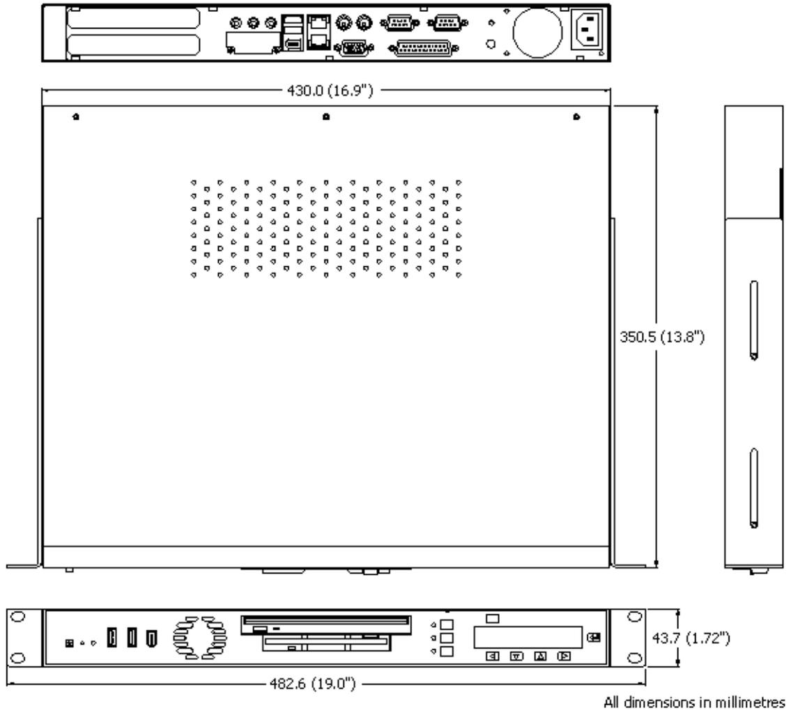
The unit complies with standard (IEC 60297 and IEC 60917) 19" Rack Mounting dimensions and will fit into a standard rack cabinet.
