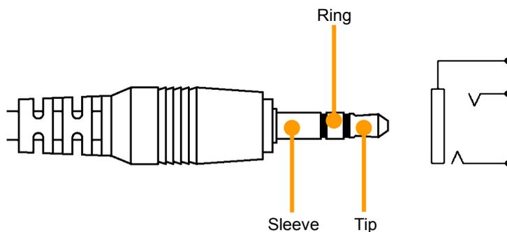
The pin settings for each connector are described in the following sections:
