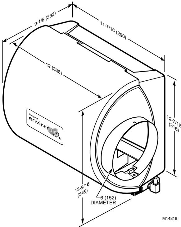
Fig. 1. Dimensions of HE225A,B in in. (mm).
