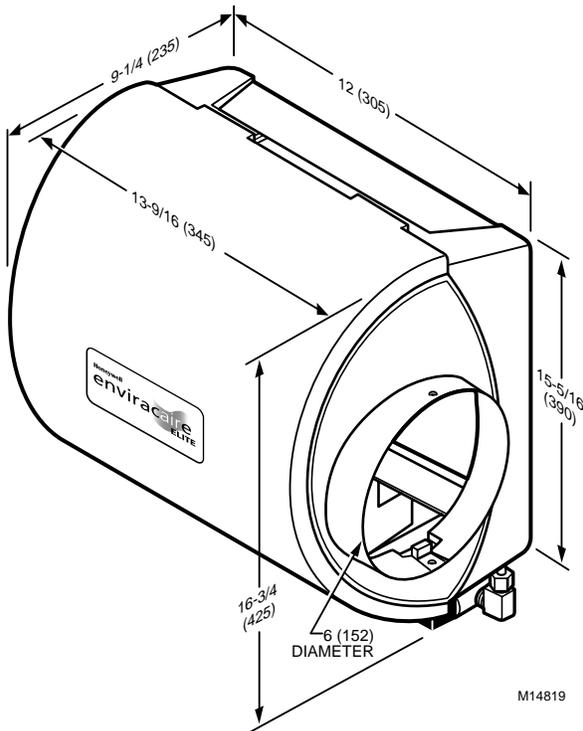
Fig. 2. Dimensions of HE265A,B in in. (mm).
