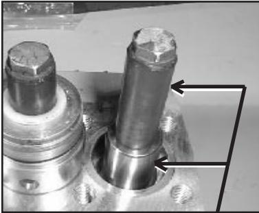
9) Check surfaces of plunger pipe (16B).
