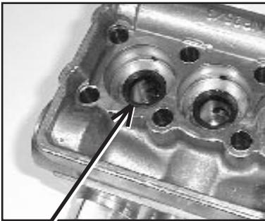
13) Generously lubricate v-sleeves. Assemble spacer rings (23A), and v-sleeves (23) into valve casing (26).
