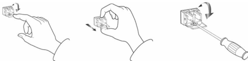
Figure 24 -- Removal of a Bale Clasp SFP Module
