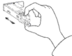
Figure 17 -- Insertion of a Mylar Tab SFP Module
