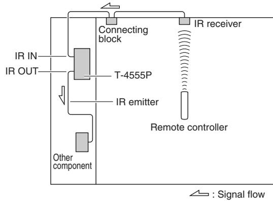
Connect the IR emitter to the T-4555P's IR OUT, and place the IR emitter in front of the other component's remote control sensor (usually located on its front panel), as shown below. See the instructions supplied with the IR emitter.
