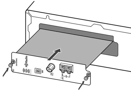
When the board meets the internal connector, apply a little more pressure so that the board plugs fully into the connector. Make sure the board's panel is flush with the T-4555P's rear panel.
