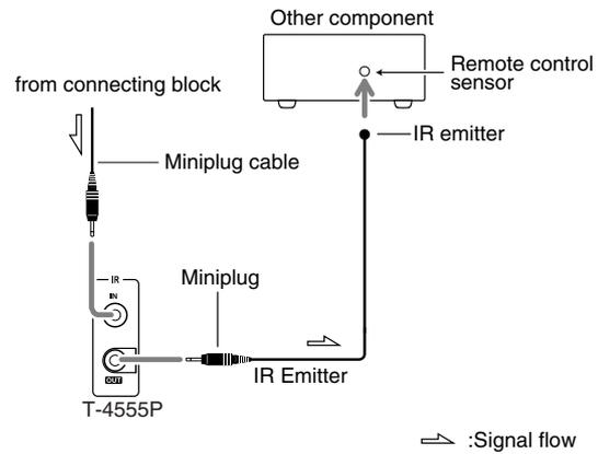
Only remote controller signals received by the T-4555P's IR IN are fed through to the IR OUT. Signals picked up by the T-4555P's remote control sensor are not output.
