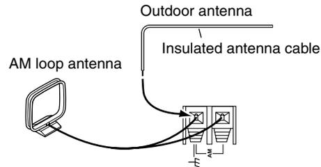
Outdoor AM antennas work best when installed horizontally outside, but good results can sometimes be obtained indoors by mounting horizontally above a window. Note that the AM loop antenna should be left connected.
