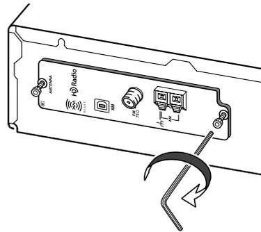
Be sure to fully tighten the screws. If they are loose, the ground connection between the board and the T-4555P may be inadequate, resulting in noise or failure.
