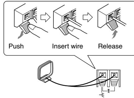
Once the T-4555P is ready for use, you'll need to tune into an AM radio station and adjust the position of the AM antenna to achieve the best possible reception.
