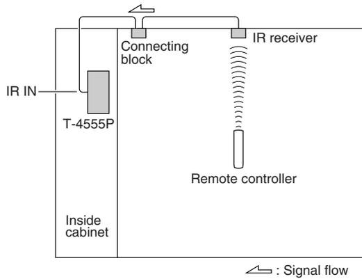
Connect the IR receiver to the T-4555P as shown below.
