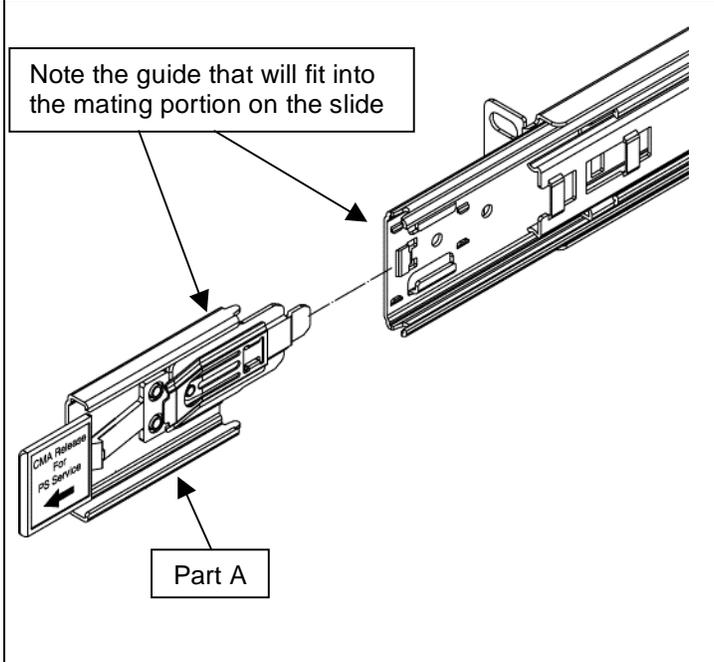
3. Connect Part B to the inside right hand side slide member by sliding it into place. A “click” will be heard once it is secured. The Cable Management System is designed to have the cross-support beam on the bottom...not the top.
