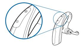
6 To end the test call, press the call control button on the headset.
