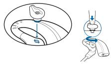
**NOTE** When installing a gel tip, ensure the raised part of the ear tip is pointed towards the curved section of the headset as shown.
