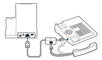
**NOTE** If your phone has a built-in headset port, you should only use the headset port if you will not be using the HL10 lifter. In this configuration, you must press both the headset button on your phone and the call control button on the headset to answer or end calls.
