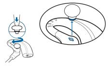
2 Choose the size and style of ear tip that fits most comfortably. Align ear tip tabs with notches in headset. Push in firmly and twist ANTI-clockwise.
