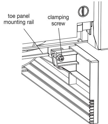
9. Close the drawer. Check that there is 1/2" (12.7 mm) minimum clearance between the bottom edge of the toe panel and the floor.
