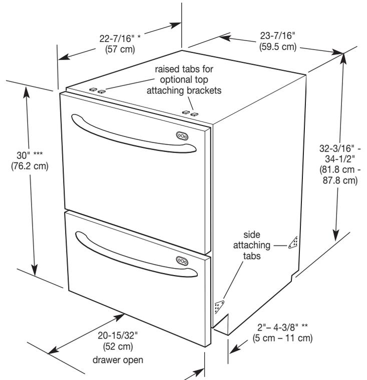
\* If custom wood panels are to be used, the product depth is specified with an 11/16" (18 mm) door panel thickness.
