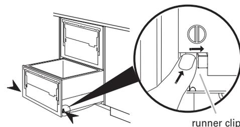
4. Lift the right edge of the drawer off its runner. Slide that runner back into the dishwasher.
