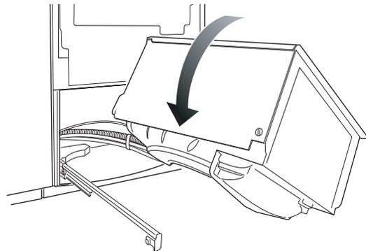
15. Make sure both runner clips have snapped into place. If they have not, pull the runner clips forward until they do.
