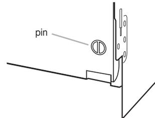
7. Gently pull the bottom of the metal plate away from the dishwasher, and then pull down.
