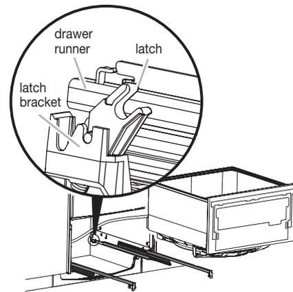
14. If the bottom drawer was rotated, rotate the drawer to unwind the hoses and then put the drawer on the runners, making sure the hoses are looping upward.
