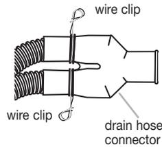
**NOTE:** The drain hose connector must not support the weight of excess hose length. Keep hoses as fully extended as possible.
