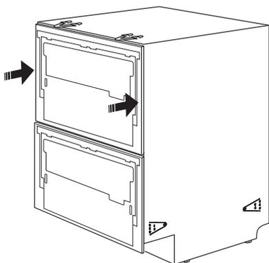
22. As the dishwasher is being pushed into the opening, slowly pull the inlet hose and drain hoses through the utility hole. Let the house wiring gather behind the dishwasher.
