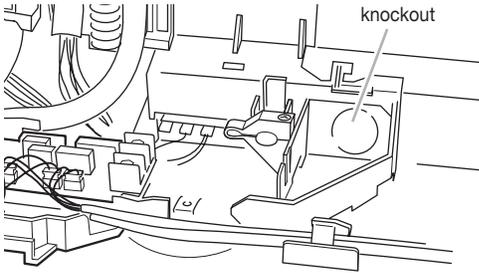
7. Run the house wiring through the conduit connector (not supplied) and into the dishwasher through the knockout opening.
