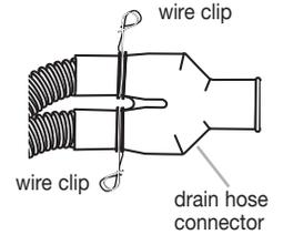
**NOTE:** The drain hose connector must not support the weight of excess hose length. Keep hoses as fully extended as possible.
