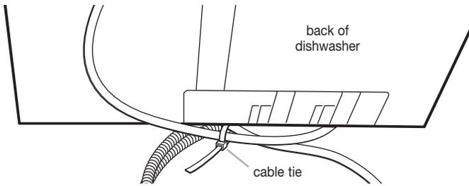
18. Completely remove the power supply cord and save it, in case a power cord installation is needed in the future.
