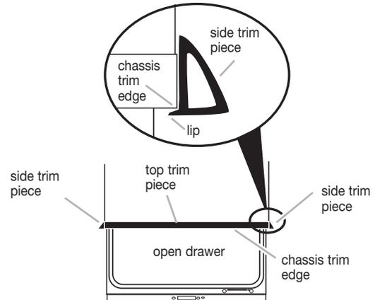
3. If using the optional top attaching brackets, place the trim pieces under the attaching brackets.
