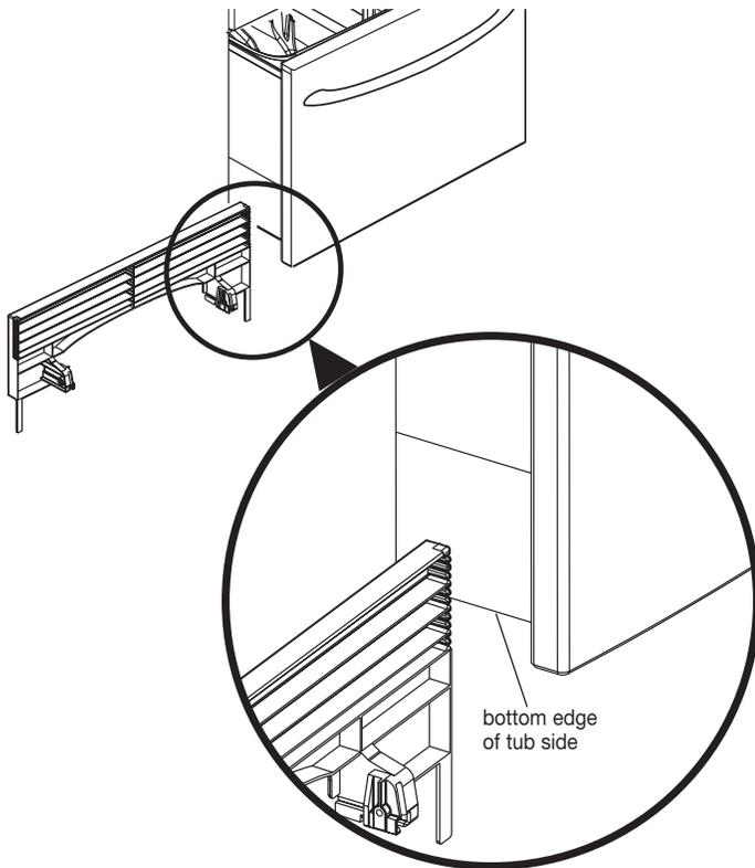
4. On a stable surface, place toe panel on a wooden cutting board and pick the closest groove to the mark. If the mark is between two grooves, choose the groove that makes the toe panel the shortest.
