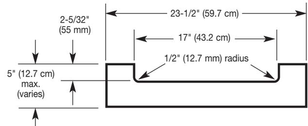
The black prefinished toe panel can also have a custom front panel with a thickness from 3/8" to 3/4" (9–19 mm) attached to it. Determine the height of the toe panel custom panel: The minimum height is 2-3/4" (70.5 mm). Measure from the top of the adjacent cabinet door front to the floor. Subtract 28-15/32" (72.3 cm) for needed toe panel height.
