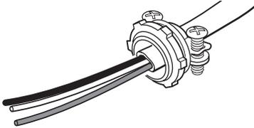
8. Secure the conduit connector in the knockout opening.
