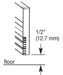
10. Slide toe panel back onto mounting rails.
