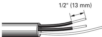
10. Insert the black supply wire and the white neutral wire into the appropriate wire clamp on the terminal block. Securely tighten the clamps.
