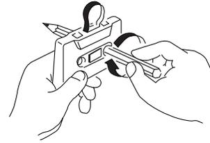
**Use a pencil to take up the slack and rotate it in the arrow direction.**
